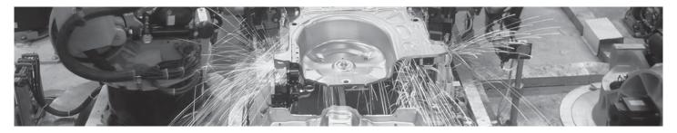
Reduce downtime with accessories that protect sensors, cables and associated components against the challenges of welding environments. Mounting brackets with ceramic coating resist accumulation of weld spatter and so reduce the need for cleaning.
