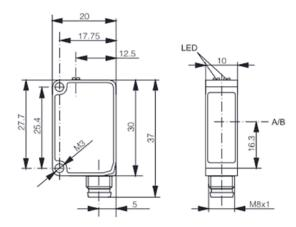
A: emitter axis B: receiver axis
