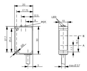
A: emitter axis B: receiver axis
