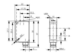
A: emitter axis B: receiver axis
