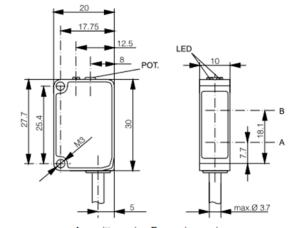
A: emitter axis B: receiver axis
